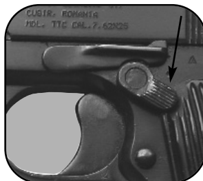
Safety lever in the downward “FIRE” position dimple/stamped dot on receiver visible.
