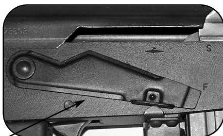
Safety lever in lower or “FIRE” position. Pulling the trigger when the safety lever is in the lower position will result in the rifle firing if there is a round in the chamber! Exercise extreme caution when handling rifle in this condition.
