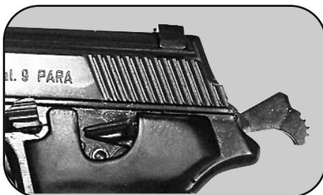
When the pistol's hammer is pulled the back off the frame, the pistol is in the “cocked” position.
