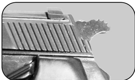
When the pistol's hammer is flush against frame, the pistol is in the “de-cocked” position.
