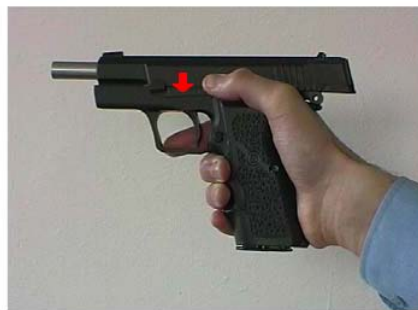
Fig. 3: Slide release from its "rear lock-up" position by depressing the slide stop
