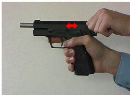
Fig. 2: Slide release from its "rear lock-up" position by cocking and releasing
