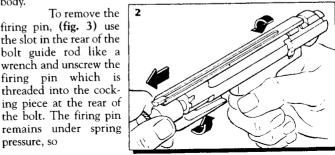
when the pin is unscrewed, care must be taken to prevent parts from springing loose when the firing pin is removed. Removal of the firing pin allows the striker spring to be removed, and it allows the cocking piece to fall free of the bolt.
