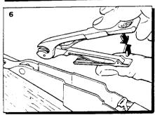
rel bands by depressing the spring keepers which hold the bands to the rifle. Next, lift off the handguard and then invert the rifle and remove the action bolts at either end. The barreled action now will lift out of the stock, and the bottom metal consisting of the entire magazine / trigger guard assembly can be removed from the stock. Reassembly is the reverse procedure. There should be no particular tricks needed to take the rifle apart and to reassemble it.
