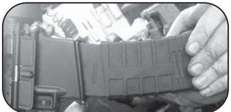
Press the magazine release button to remove the magazine from the rifle.
