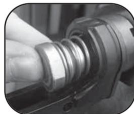
16. With a punch, remove the extractor pin from the bolt assembly. (See Illustration #25.)
