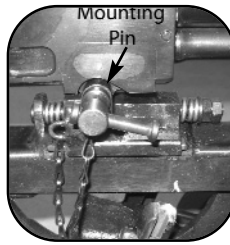
Mounting pin locked into place.
