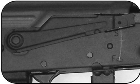
Safety lever in upper "SAFE" position. The lever will be above or covering the stamped letter "S" on the receiver.
