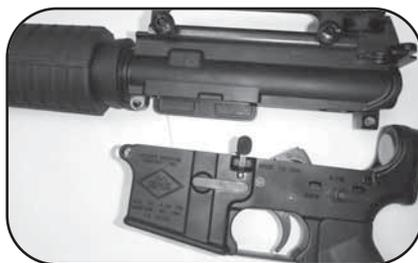
8. Pull charging handle to rear and remove bolt and carrier assembly. (See Illustration #16.)
