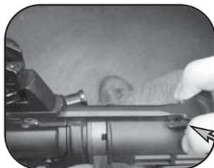
**Charging Handle:** Located at the rear of the receiver, used for operating the bolt. Depress the charging handle lock located on the left side of the firearm and pull back on the charging handle to move the bolt to the rear. (See Illustration #5.)
