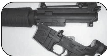
6. Press the front pivot pin in from left side of lower receiver and pull out right side until it comes to a positive stop. (See Illustration #14.)
