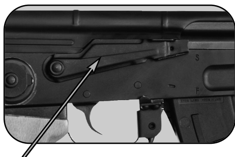
Safety lever in upper “SAFE” position.
