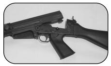
Removing the Receiver Cover
