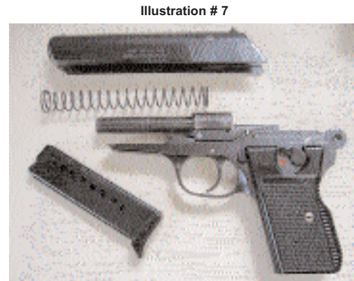
The Century Czech Model 70 pistol disassembled into its major component parts groups. No further disassembly is needed for routine maintenance.
