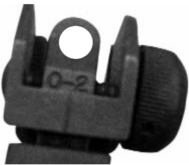
Rear Sight Aperture (center) Windage Adjustment Knob (right)
