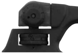
Elevation Knob (at bottom) Windage Knob (at top)
